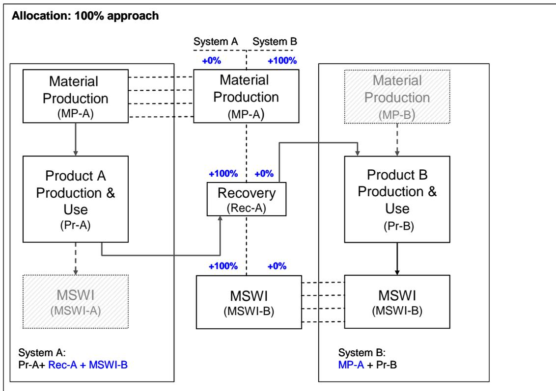
Figure 9: Principles of 100% allocation (schematic flow chart)
