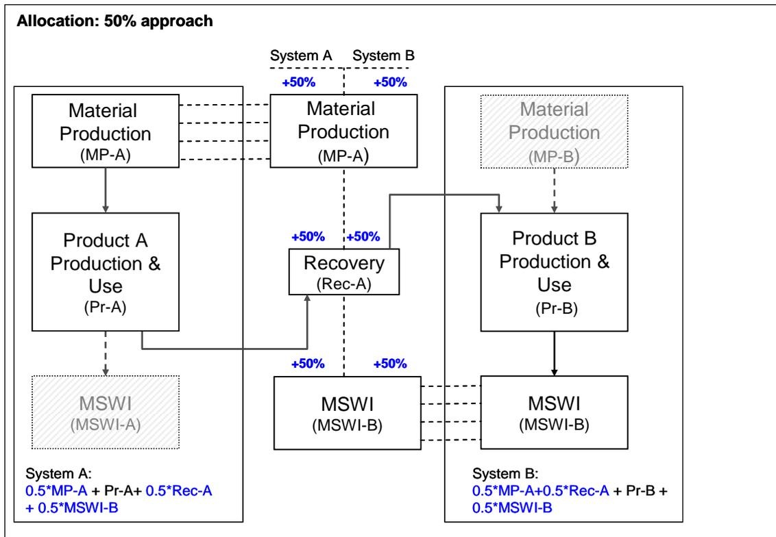
Figure 8: Principles of 50% allocation (schematic flow chart)
