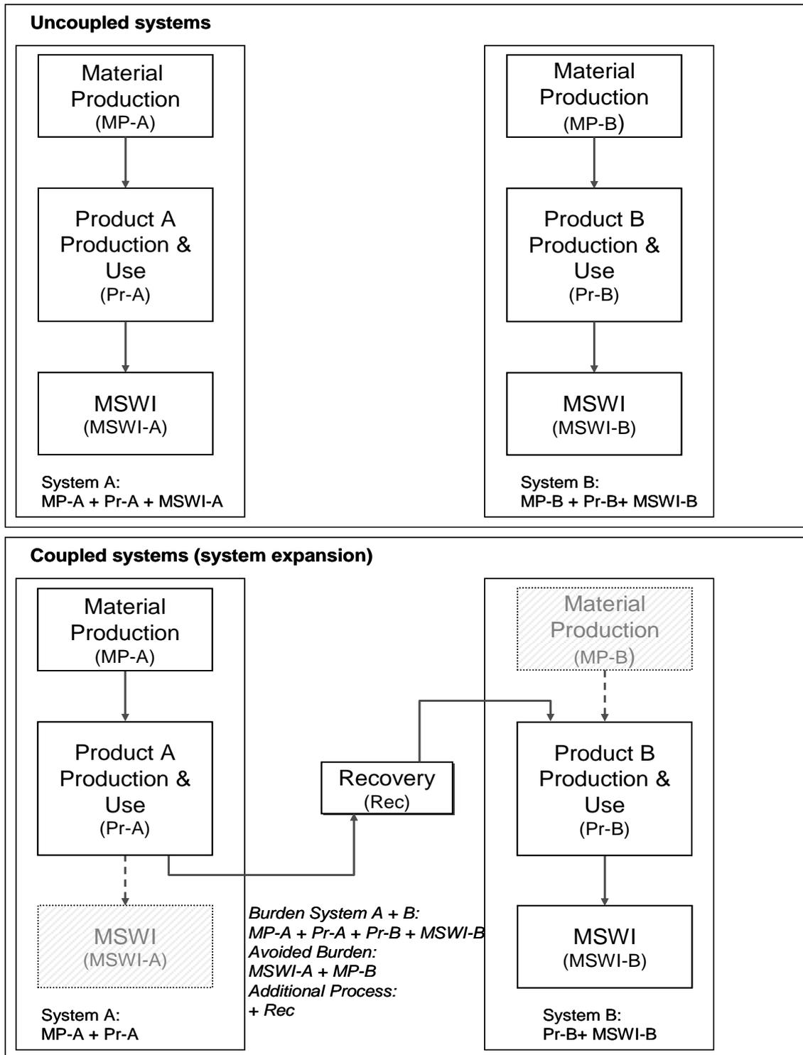
Figure 7: Additional system benefit/burden through recycling (schematic flow chart)
